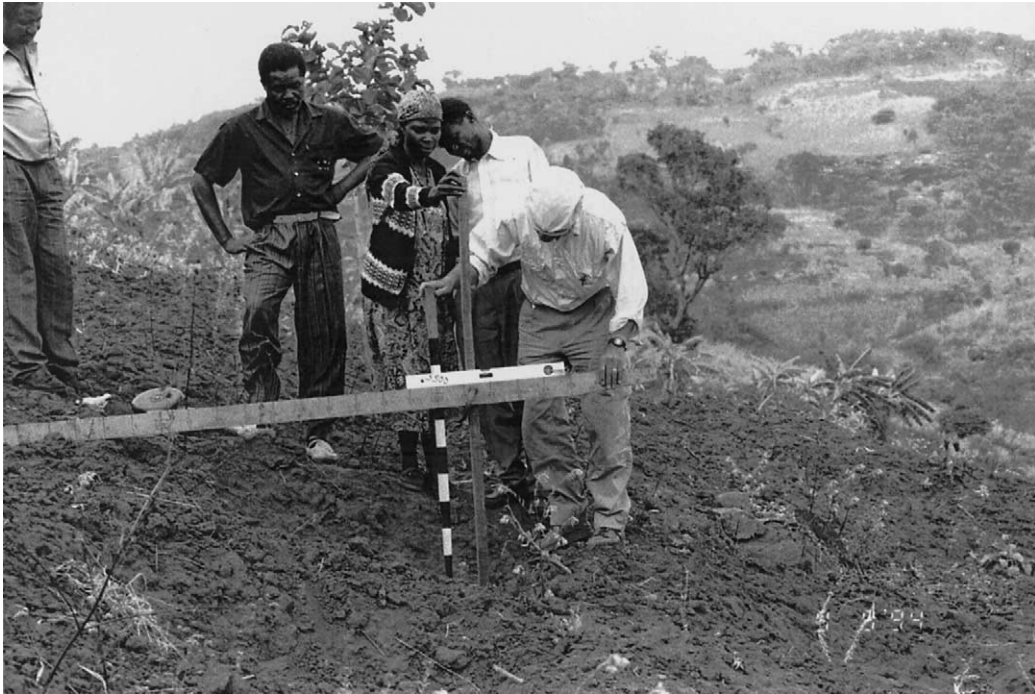
Fig. 2. Measuring the soil surface profile of ngoro conservation structures at an on-farm site in Mbinga District, Tanzania. The conservation structure profile gauge, depicted here, has been designed and developed by the Environment Research Project Team to reliably measure, monitor and compare soil surface profiles (SSP).
