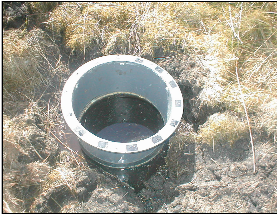
Figure 8 . Collar and a cylindrical chamber in a hollow; a circular rubber was used to make a tight seal around collar and chamber.
