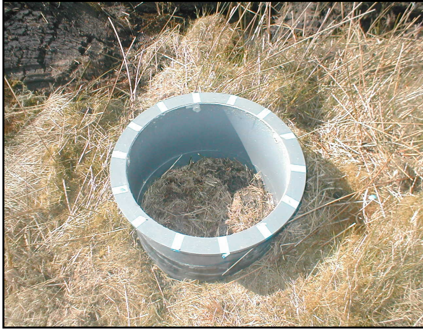
Figure 7. Collar and a cylindrical chamber on undistributed ground; a circular rubber was used to make a tight seal around collar and chamber.
