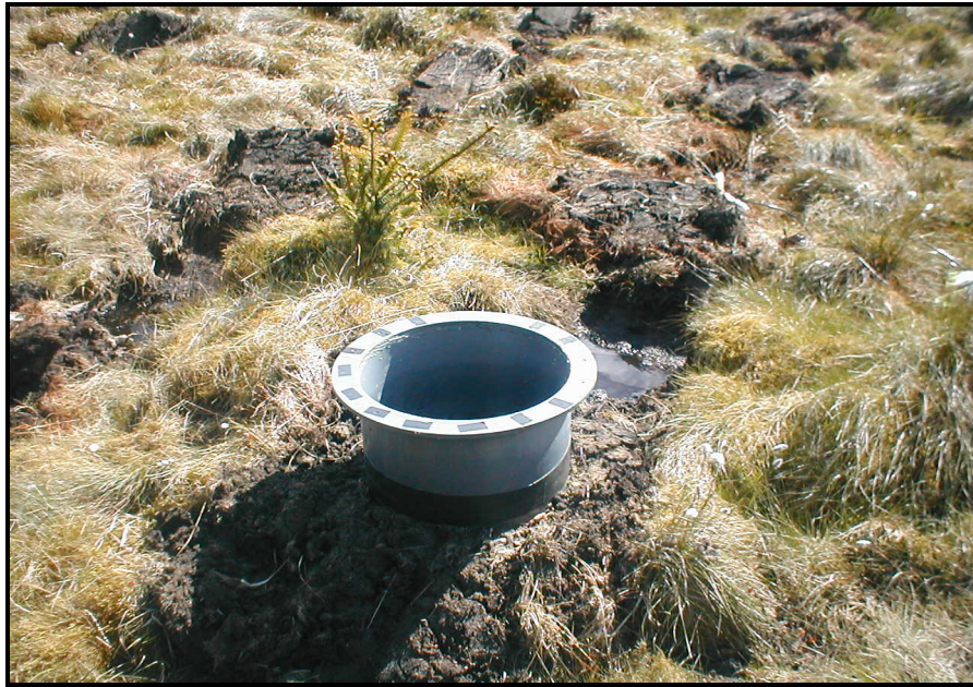
Figure 9. Collar and a cylindrical chamber on a mound hollow; a circular rubber was used to make a tight seal around collar and chamber.
