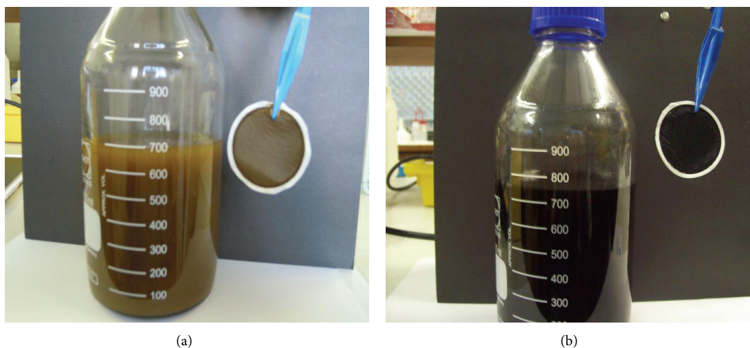
FIGURE 1: (a) Brownish graphene oxide and (b) blackish reduced graphene oxide.
