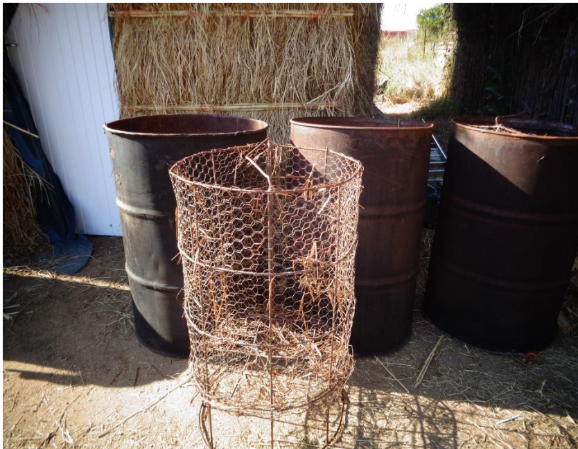
Figure 7: Mesh wire cage and drums used for steaming substrate
